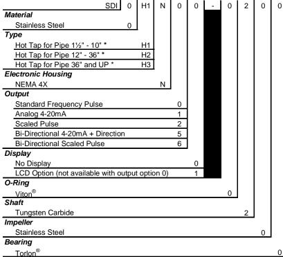
\* Pipe Sizes for reference only - Depending on pipe material, tapping saddle, or existing hardware longer sensor length may be required - Contact Factory.
